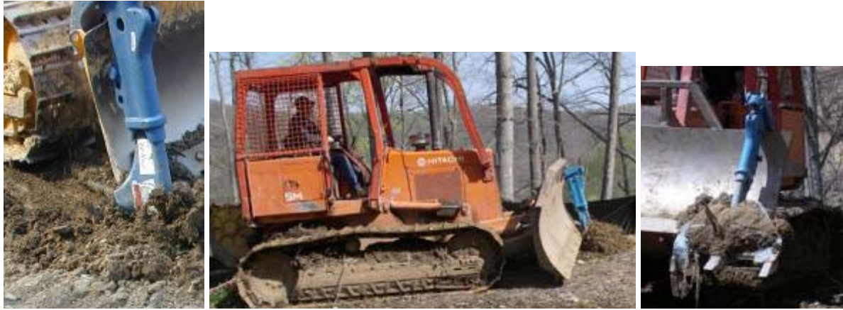
Figure 5. Modified ripper-tooth dozer-blaze assembly
