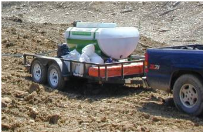
Figure 6. 500-gallon log landing hydroseeder mounted on a trailer to be pulled behind a truck.
