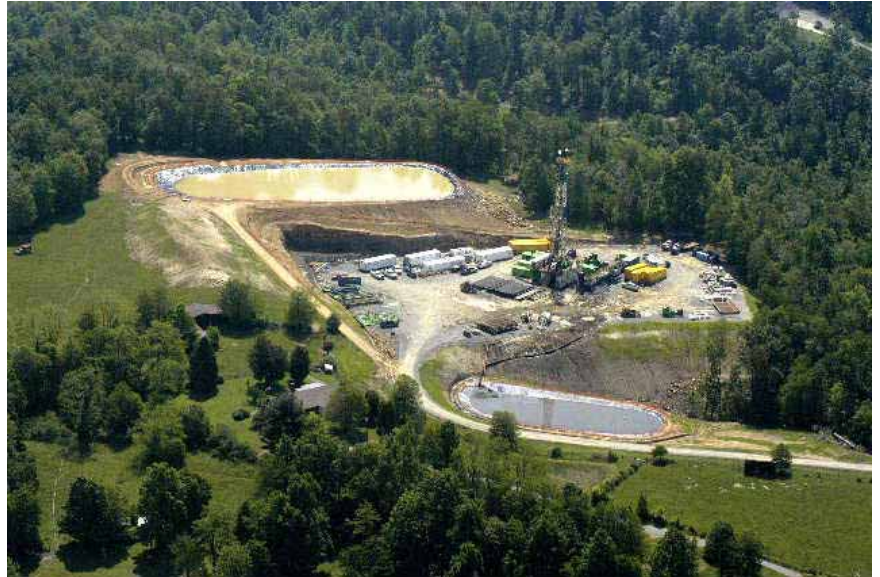
Well site during active drilling to the Marcellus Shale formation in Upshur County, West Virginia. (An additional water storage pit is not in the photo.) Copyright WV SORO, June 2008.
