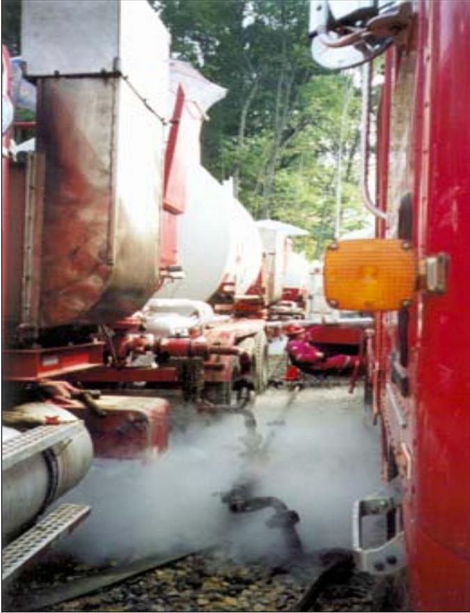
Figures 4-1 and 4-2. Liquid nitrogen tanker trucks transport gas to the site for nitrogen foam fracturing. Nitrogen will travel through pipes to be mixed with water and a foaming agent at the wellhead prior to injection. The foam is used to create and propagate the fracture deep within the targeted coal seam.
